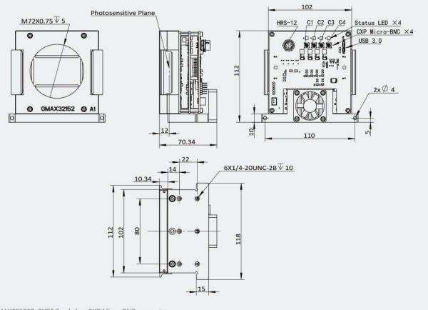
Note: HBW-GMAX32152S-CXP2.0 only has CXP Micro-BNC connector, HBW-GMAX32152S-U3V only has USB 3.0 Micro-B connector.
